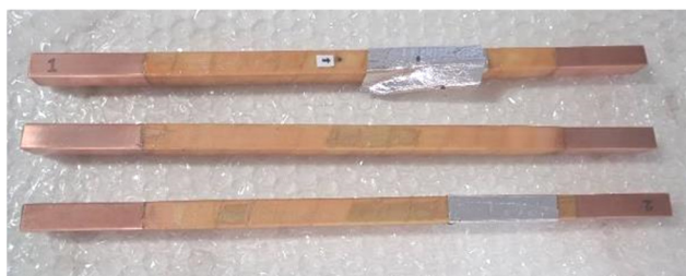
Figure 1: Photograph of Cyanate-ester prepreg tapes after wound on hollow conductors and cured.
