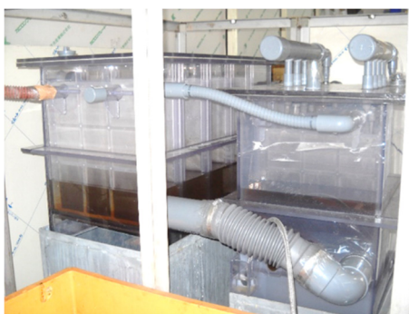
Figure 2: A photo of improved EP acid tank.
