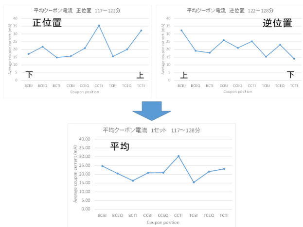
Figure 5: Average coupon current of one forward position VEP (upper left), one reverse position VEP (upper right), and one F-R cycle (lower).
