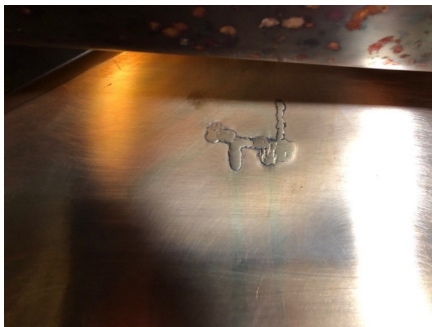
Figure 7: Resonator for RRC repaired in June 2020.
