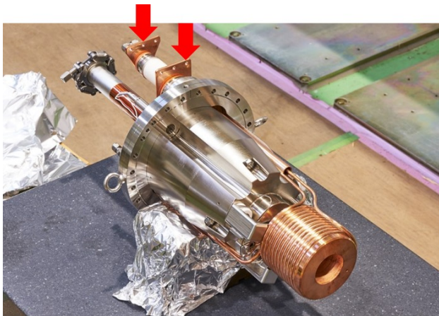
Figure 2: Flux Concentrator (FC) mounted on a vacuum flange with several components. Red arrow shows electrical connection point to the FC.
