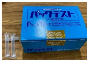
Figure 6: Pack test used for the measurement of  $\text{H}_2\text{O}_2$  concentration.
