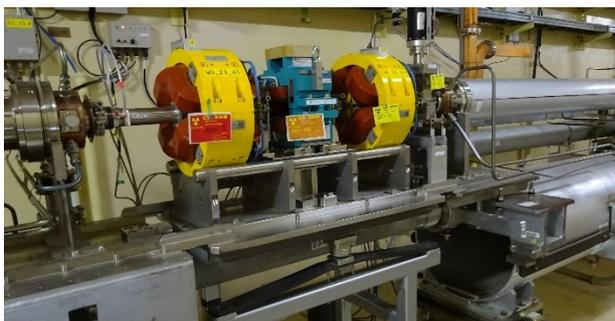
Figure 4: Pulsed steering between DC quadrupole magnets at Sector 2.
