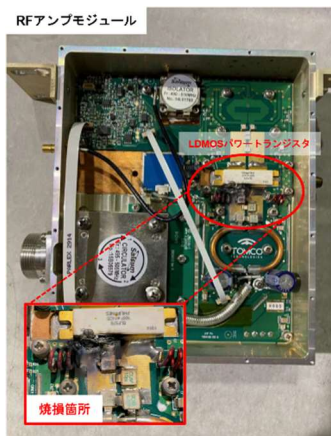
Figure 3: Burnout in RF amplifier module of booster synchrotron.
