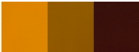
Figure 3: The film on the left has zero dose, and the film on the right has more dose.
