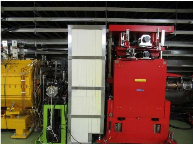
Figure 8: Polyethylene Shield for the Protection of Beam Injection Kickers.
