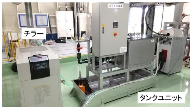
Figure 3: The tank unit and the chiller.
