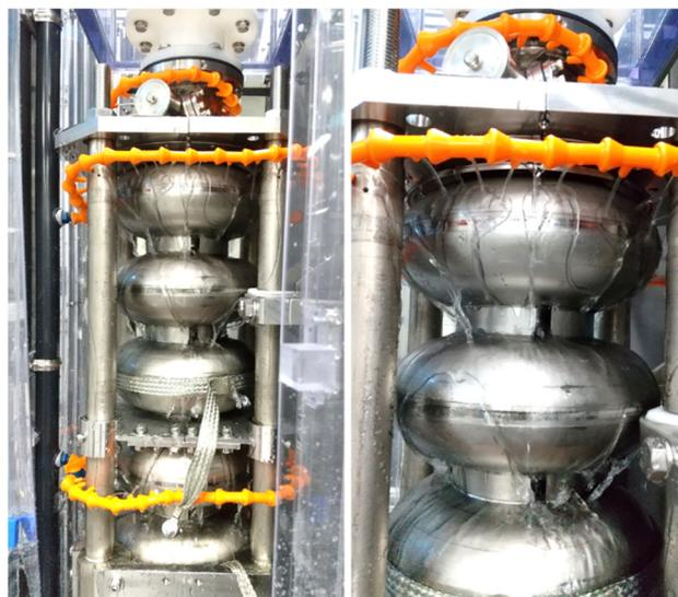
Figure 8: Cooling water shower to a 9cell cavity.
