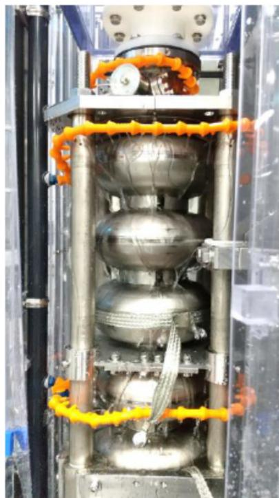
Figure 6: Cavity water cooling system using pure water.
