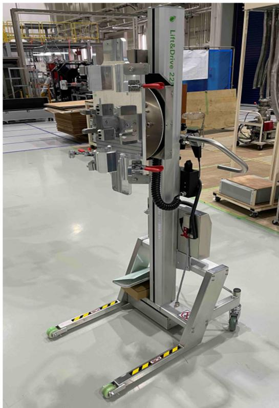
Figure 8: Lifter for cavity transport.
