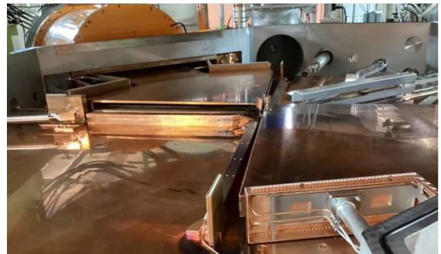
Figure 1: Inside of the AVF cyclotron chamber. Two dee electrodes can be seen.
