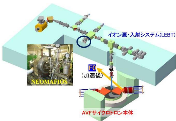
Figure 1: Schematic of ion source and LEBT at RCNP.
