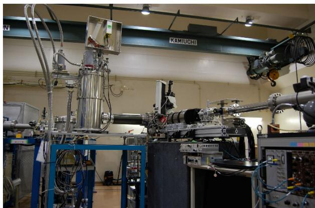
Figure 7: Photo of the STJ detector for the SC-PIXE.
