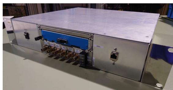
Figure 6: Picture of the prototype cavity driver module.
