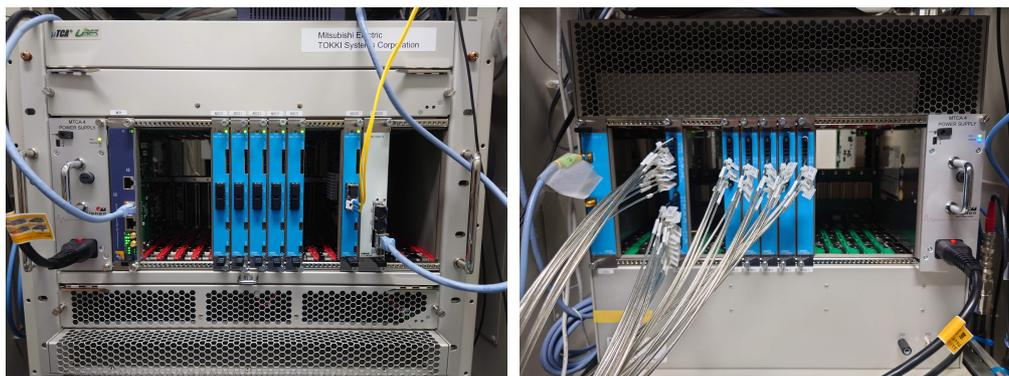
Figure 9: The photo of the developed LLRF control system. (Left: AMC side. Right: RTM side. )
