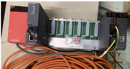
Figure 5: Mitsubishi PLC inside Coil Power Supply controlled by another PLC CPU using NetDEV.
