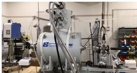
Figure 4: Photograph of GM cooled 6T solenoid.
