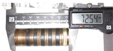
Figure 3: A stacked  $MgB_2$  array for the undulator prototype.
