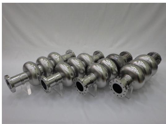
Figure 2: 3-cell cavities; KEK-R16, R16b, R17 and R17b (from left to right).
