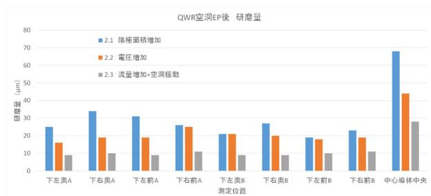
Figure 9: Removal thickness of the cavity after each EP.
