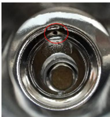
Figure 6: A photo of a hole in the center conductor.
