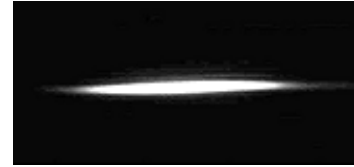
Fig. 4: Qualitative image of the electron beam observed by a focusing system.
