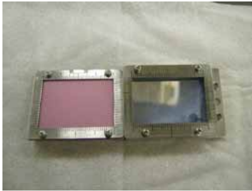
Figure 2: Screen folder mounted with both of a ceramic screen and a Cherenkov radiator. The left screen is a profile monitor with a fluorescence ceramic screen with a thickness of 0.1 mm and it is tilted vertically by an angle of 45°. The right screen is the aerogel radiator and it is tilted of 55.8°.
