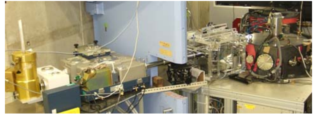
Fig. 2 FIR beam line attached to the 6 MeV MIRRORCLE in the right. FTIR and Si bolometer are seen in the left. Whole system is under the vacuum.
