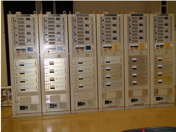
Fig. 3. Driver amplifiers for MR.
