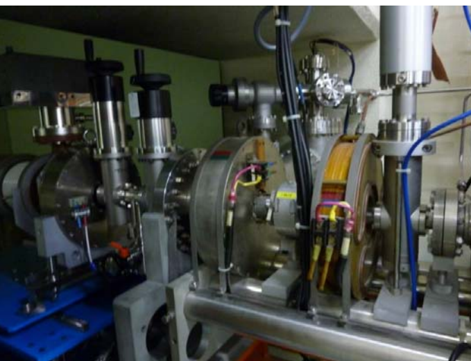
E-gun with dual vacuum valves
