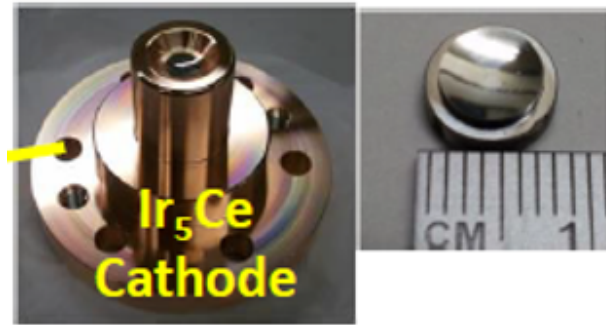
Ir 5 Ce Cathode QE=1 × 10 -4 @266nm Long lifetime
