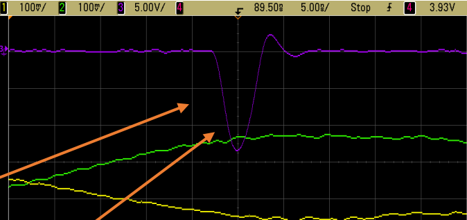
Beam current of 300 mA in the end of accelerating structure, duration is 2.5 ns (half of pulse), energy is about 4 MeV
